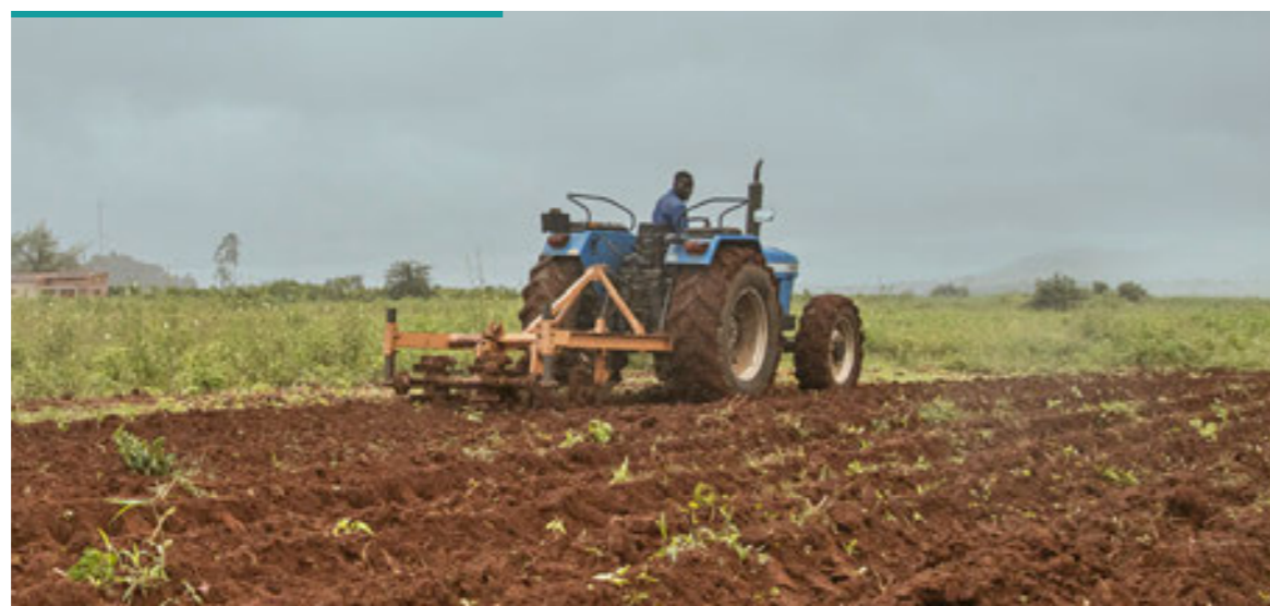
Farmer preparing land using minimum tillage technology (mechanical ripper) introduced by PROMAC
